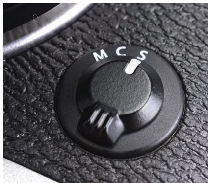
▲ Selector on the front panel switches between the focusing modes.
