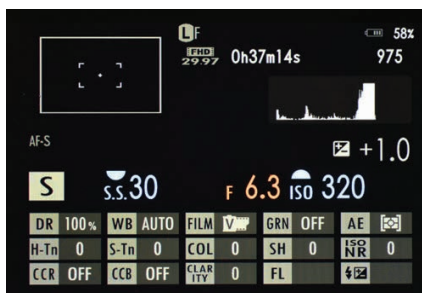
▲ Monitor-based 'Info Display' includes a large selection of function settings, the exposure settings, a real-time histogram and an AF point/zone map.
