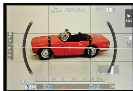
▲ Live view screen is configurable with an extensive choice of elements and read-outs, including a real-time histogram, a highlight warning, either single- or dual-axis level indicators and a choice of grid patterns.
