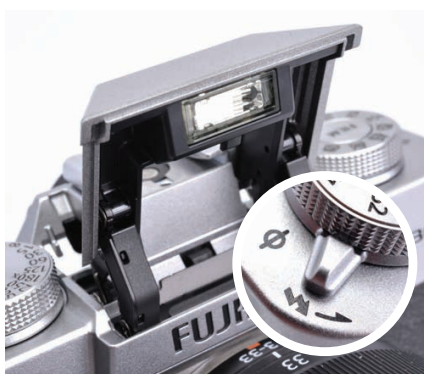
▲ Pop-up flash is activated via a lever below the 'Film Simulation' dial. Flash power is GN 7.0 at ISO 200.
