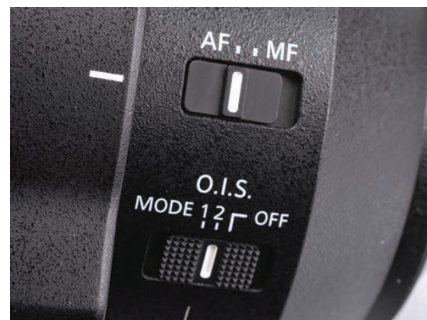
▲ On-barrel controls are a focus limiter, AF/MF switch and optical image stabiliser mode selector.
