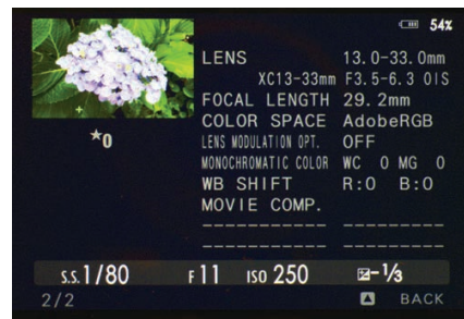
▲ Review/replay screens include a full set of histograms and two pages of capture data, including the lens settings.
