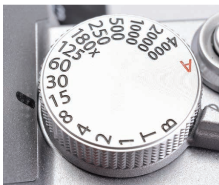
▲ Shutter speed dial is a chunky component. T setting provides access to speeds slower than one second.
