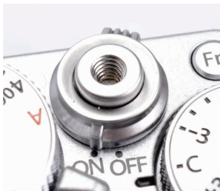
▲ Shutter release button retains a cable release socket.
