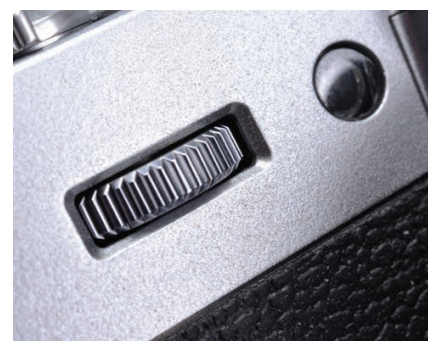
▲ Both the front and rear input wheels have press-in actions for various functions. The front control cycles through a selection of adjustments – apertures, ISO settings, exposure compensation or the 'Film Simulation' profiles
