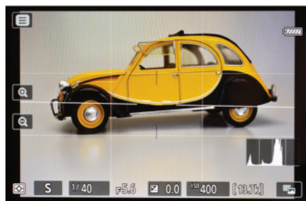
▲ Live view screen elements include a dual-axis level display, guide grid and a real-time histogram. You can cycle through up to four display designs.
