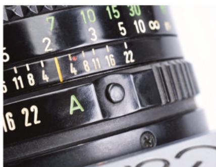
▲ Canon's FD lenses allowed for full-aperture metering from the start so adding auto aperture control was a fairly straightforward modification.
