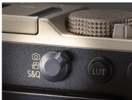
▲ Photo/Video mode switch also has a position for the 'Slow & Quick' video framing rates for recording time-lapse or slow-motion sequences.
