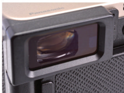
▲ Viewfinder is 1.0 cm OLED with 2.36 megadots resolution and 0.74x magnification (35mm equivalent).
