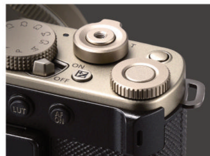
▲ Rear control wheel is a navigational tool while the 'Fn' button in its centre is extensively customisable.
