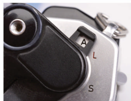
▲ Main switch has three settings – 'A' for on, 'L' for off (i.e. lock) and 'S' for engaging the self-timer which is electronically timed.
