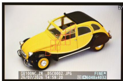
▲ Focus point selection display in replay shows you exactly what the AF system was thinking.
