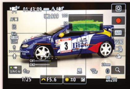
▲ Waveform monitor displays are available in luminance-only line (left) or RGB types. Waveform displays assist with determining the overall brightness of a video picture similar to the brightness/RGB histograms for stills.
