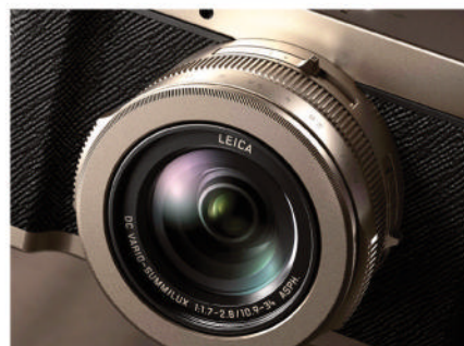
▲ Leica-endorsed DC Vario-Summilux 10.9-34mm f/1.7-2.8 zoom is equivalent to 24-75mm.
