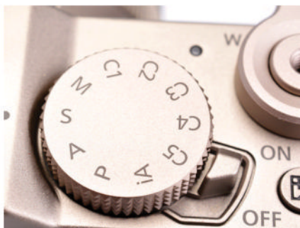
▲ Main mode dial has five positions for storing customised camera set-ups.
