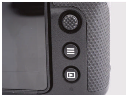
▲ Rear control panel comprises just three buttons... the important one is the menu access button in the centre.
