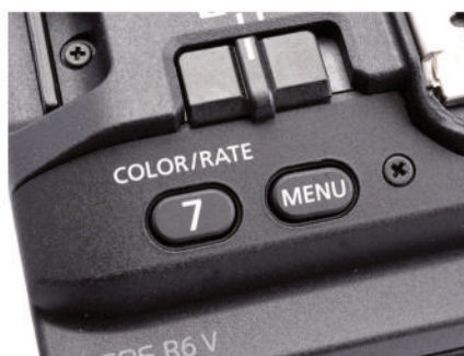
▲ The 'Color' capture function for the 'Rate' button gives direct access to the 'Picture Style' and 'Colour Filter' menus, by-passing the main menus.
