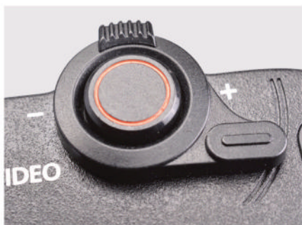
▲ Shutter release – which is also the video/stop start button – includes a power zoom lever.
