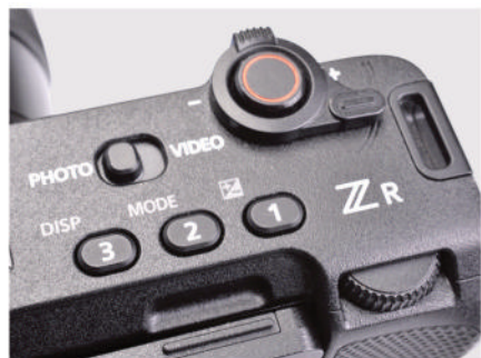
▲ External controls are kept to a minimum, but just about everything can be customised. The 'Fn2' button's default is exposure mode selection.
