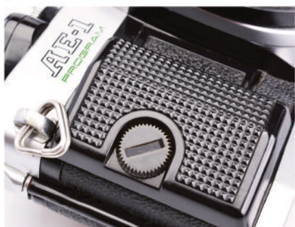
▲ On the AE-1 Program, Canon turned the front compartment battery cover into a small handgrip. It does improve the handling.
