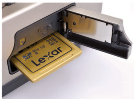
▲ Memory card has its own compartment in the camera's base.
