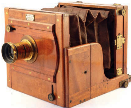
The English Collins Half-Plate Tailboard camera, c.1890, was typical of the kind of cameras that used dry plates
