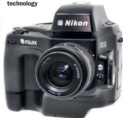
Two early attempts at building DSLRs: a Kodak DCS 410 , which mounted Kodak digital technology on a Nikon N90 SLR (left), with a Nikon E2 , made more bulky than most to allow room for its reduction optics technology
