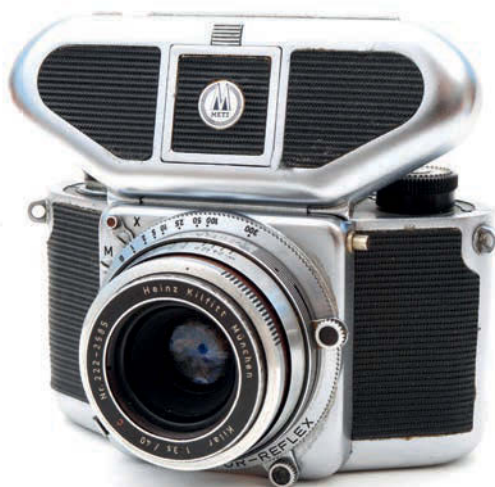
The Mecaflex was an unusual miniature SLR from 1953 that shot 24x24mm pictures on standard 35mm film
