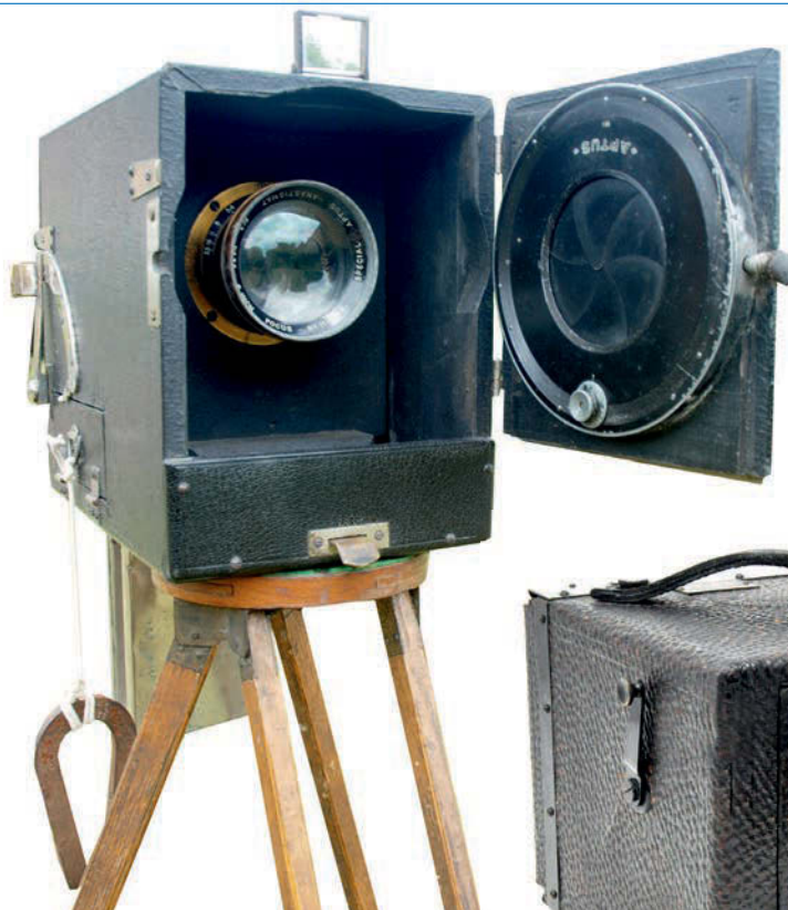
The Aptus was a while-you wait camera that shot pictures and developed them on the spot in an attached tank, all in about five minutes
