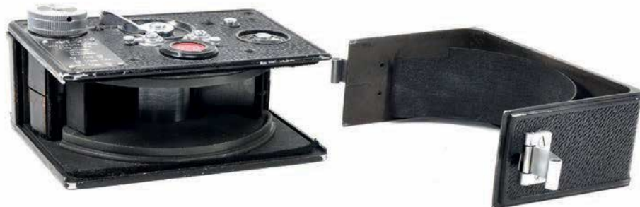
Inside the FT-2, showing its curved film path
