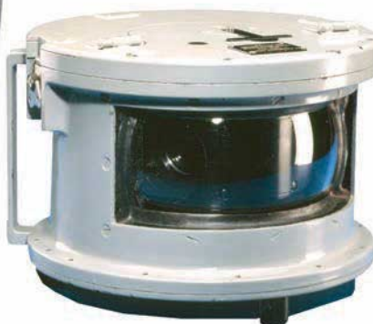
From 1950, the extremely unusual Underwater Panoramic Camera produced by Photogrammetry
