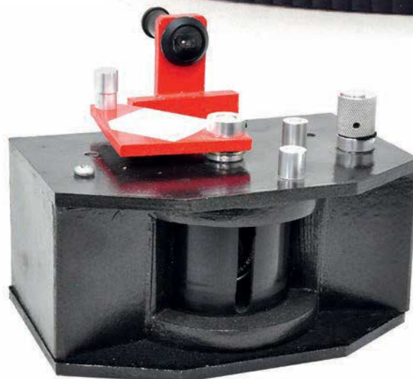
The Wideboy with its manually operated swing lens
