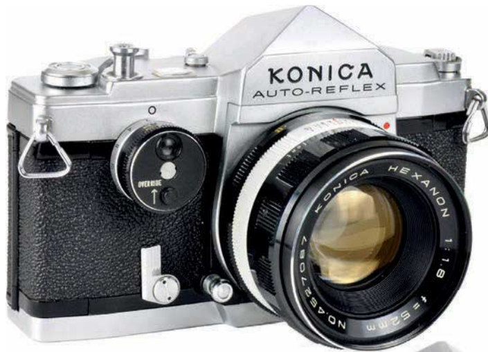
Konica Auto-reflex, unusual in offering full-frame and half-frame options on 35mm film
