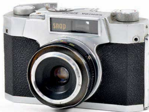
The Konica Snap, a simple viewfinder camera that predated the company's many 35mm compact cameras
