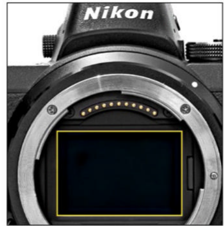
Picture 2: A full-frame sensor in a mirrorless camera that is 36 x 24 mm in size and has an aspect ratio of 3:2.
