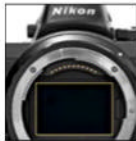
Picture 2: A full frame sensor in a mirrorless camera that is 36 x 24 mm in size and has an aspect ratio of 3:2.
