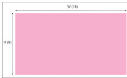
Picture 1: Aspect ratio means (W:H). As shown here, it is 16:9 that corresponds to your HDTV.
